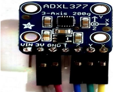
Figure 5: Triple-Axis Accelerometer (+-200g)
